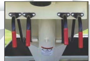
Easy Gate Control on Operator Side. 4 Controls/4 compartments-Seed Titan™ 4
