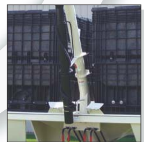
Auger Fill Tube with Lockdown System
